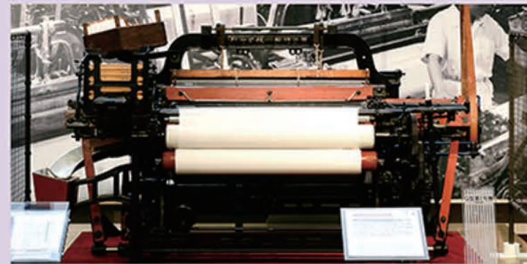
無停止杼換式豊田自動織機(G型) Non-Stop Shuttle-Change Toyoda Automatic Loom, Type G
